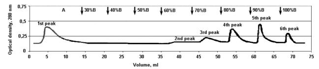
Fig. 3. Separation of different human IgG subclasses using A-protein affinity chromatography (stepwise elution): A — phosphate buffer; B — citrate buffer.
