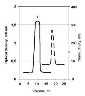
Fig. 2. Buffer change for a preparation of the human IgG by gel-filtration on a Sephadex G-25 column: I - human IgG elution from the column in the phosphate buffer; II - ammonium sulfate elution.
