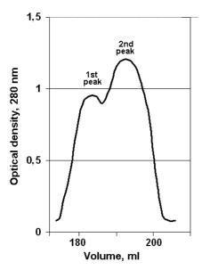
Fig. 7. Purification of the human IgA by gel-filtration on a Sephacryl S-300 column:  $1^{st}$  peak — human IgA;  $2^{nd}$  peak — human IgG.
